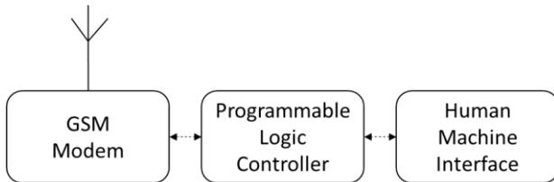
Figure 9: Display and Control Station architecture diagram.
