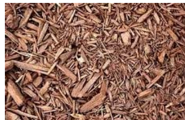
Fig. 4. CCA-treated wood chopped into smaller pieces for percolation tests
