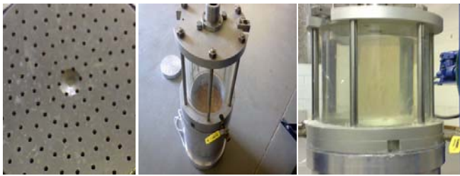
Fig. 6. (a) and (b) Perforated plate through which de-ionized water as influent in the reservoir section flowed simulating low intensity rain droplets
