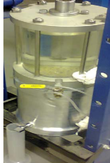
Fig. 7. Percolation test under study using de-ionized water as permeant for CCA-treated wood with the effluent collected and tested at intervals to track the concentration levels of the targeted chemical ions of concern
