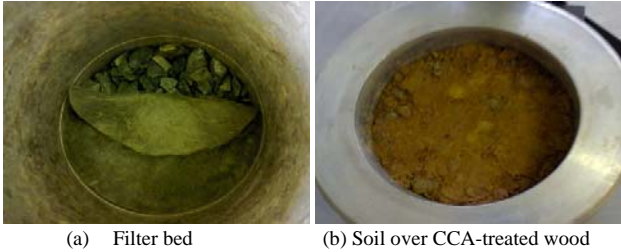
Fig. 5. (a) and (b) Wet geotextile placed over selected gravel and lightly compacted clayey soil over chopped CCA-treated wood in the bucket section
