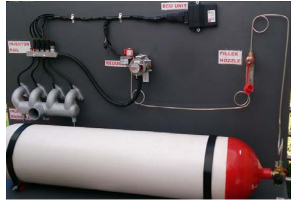
Figure 1 - Complete natural gas kit for vehicle integration
