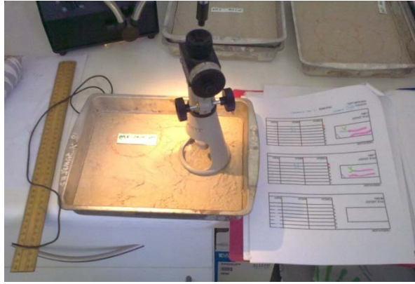
Figure 2: Measurement of crack area.
