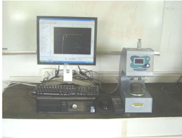
Figure 1: The Vicat apparatus in operation [5]
