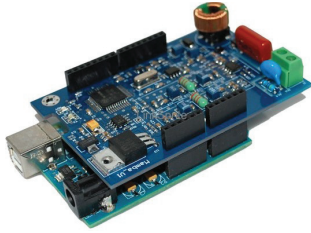
Fig. 3. Picture of Mamba Narrowband powerline communication shield.
