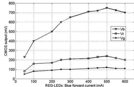
Figure 7. The CMOS colour sensor response under the influence of the light from the blue LED
