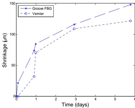
Figure 9 Shrinkage measured by the groove FBG sensor.
