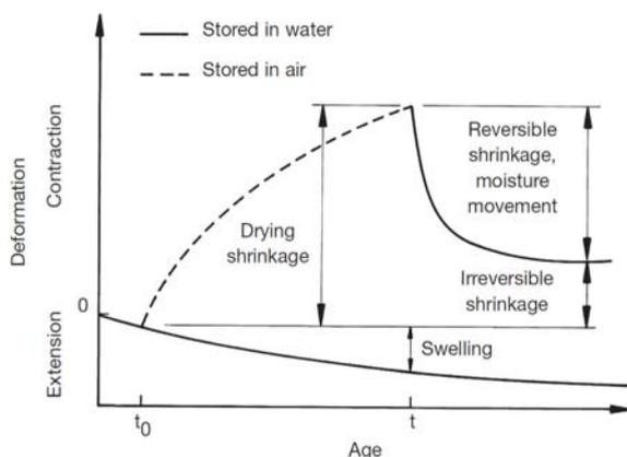
Figure 1 Moisture movement and deformation in concrete: concrete that dried from age  $t_0$  until age  $t$  and was then re-saturated [14]
