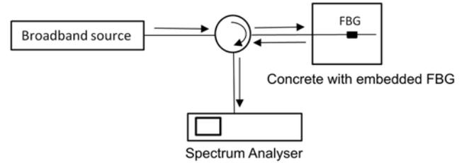
Figure 2 Optical system setup.
