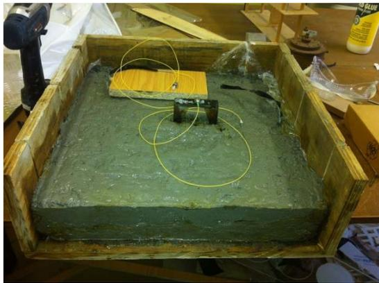
Figure 5 Completed cast with the strut sticking out of the surface, before it was removed.
