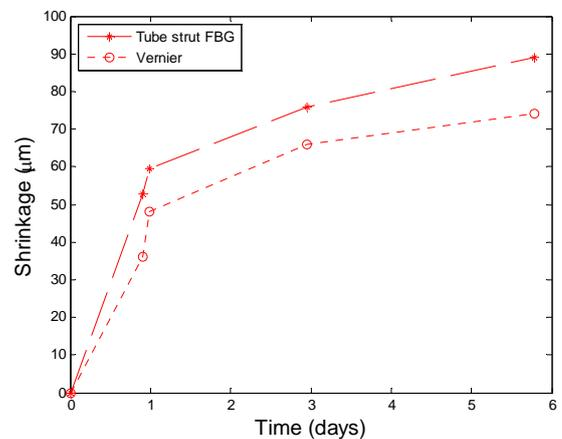
Figure 8 Shrinkage measured by the tube strut FBG sensor.
