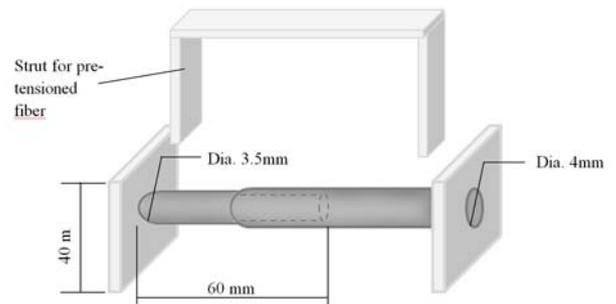
Figure 3 Tube and strut device.
