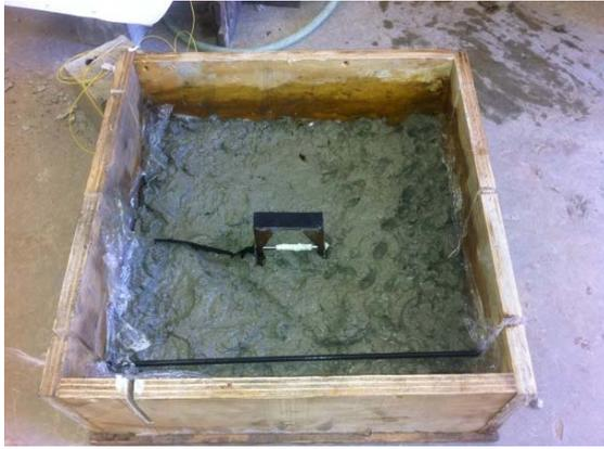
Figure 4 Tube and strut with FBG placed in wet stage concrete
