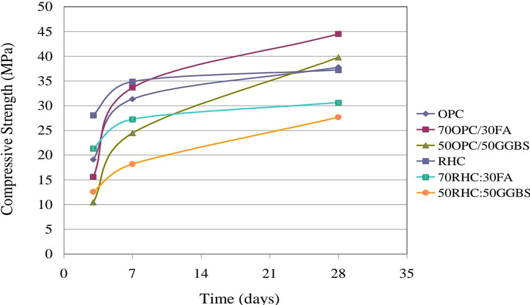
Figure 6: Strength development in OPC /RHPC /FA /GGBS concretes of equal cost of 780 R/m<sup>3</sup>
