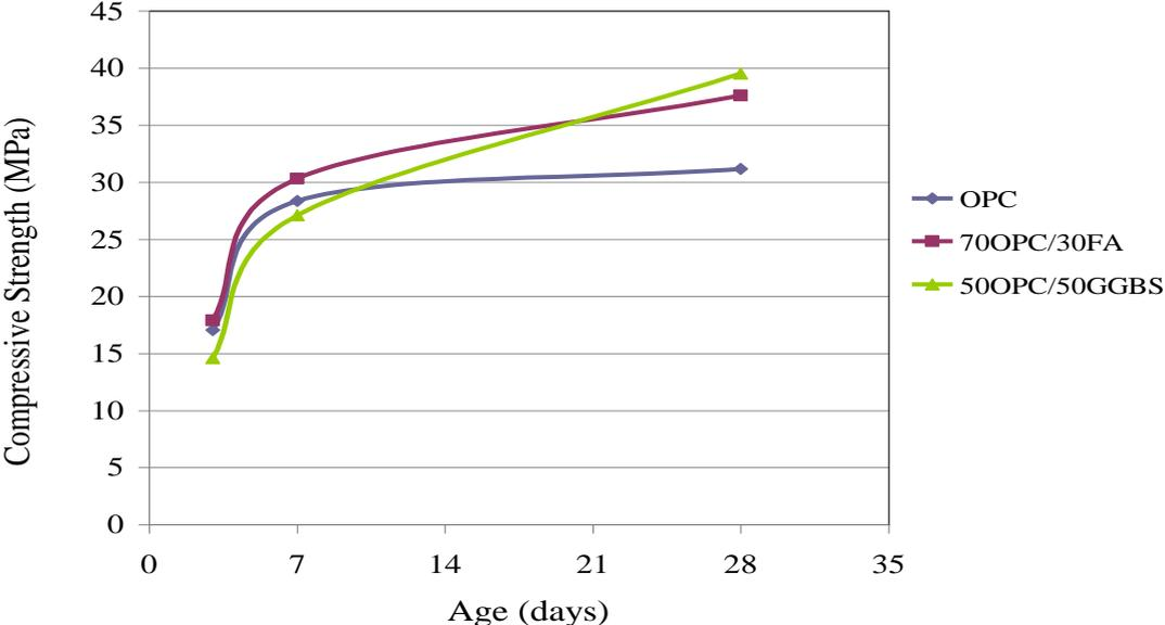
Figure 5: Strength development in OPC /FA /GGBS concretes of equal cost of 758 R/m<sup>3</sup>
