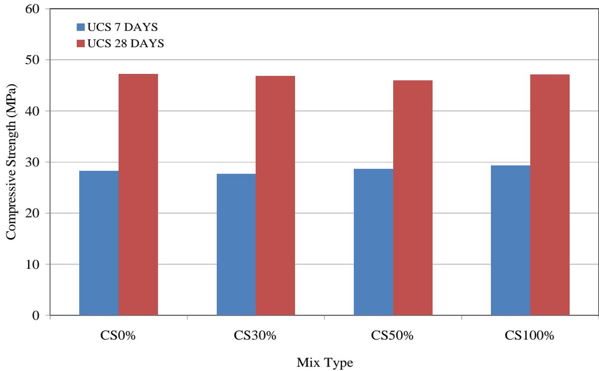
FIGURE 4 Compressive strengths of CEM I/ggbs ('CS' mix designation) concrete mixes
