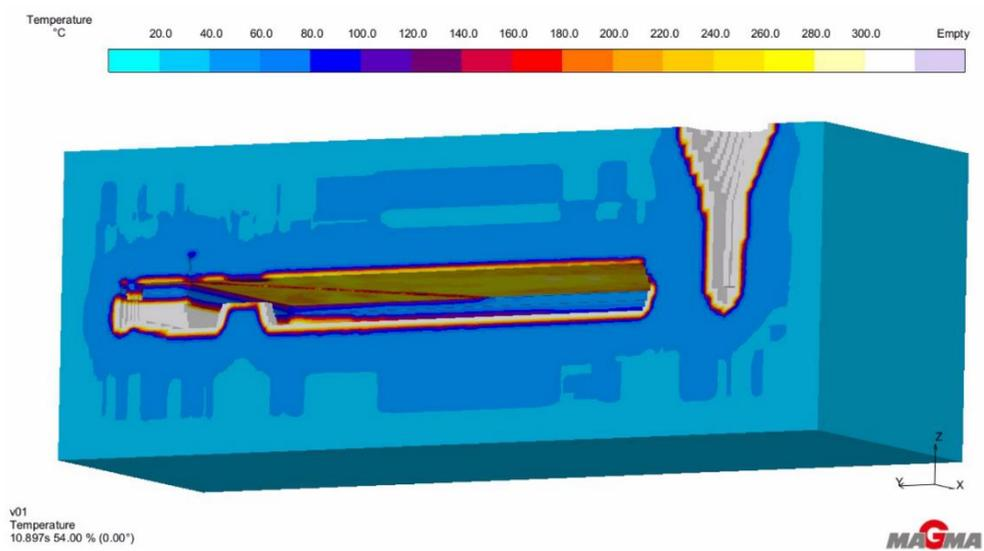
Figure 9 - Simulation data: mould temperature during filling (8-10s).
