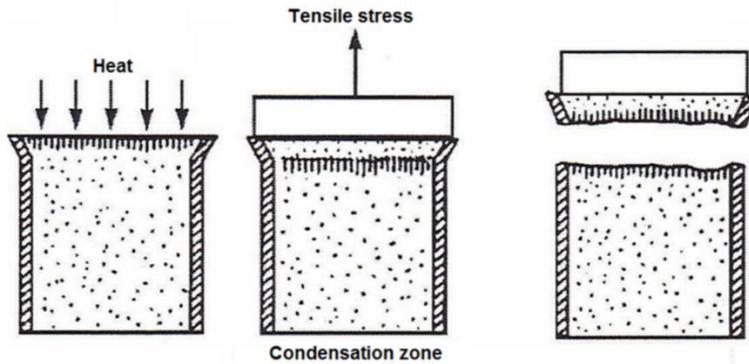
Figure 6 - Schematic representation of the wet tensile test.
