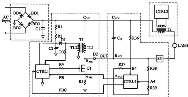
Fig. 5. Electronic ballast driver for mercury vapor lamp.
