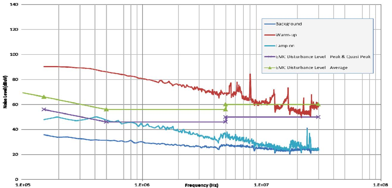
Fig. 9. Frequency domain waveforms and harmonics for 150kHz – 30MHz range (Electronic Ballast).
