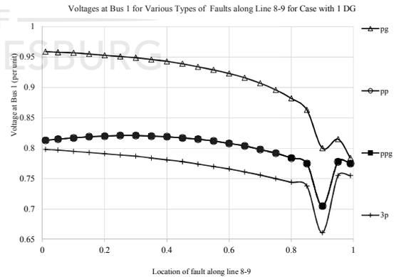
Fig. 12: Magnitude of voltage sag on the faulted phase recorded at bus 1 for faults on line 8-9 for Base Case and DG Case.
