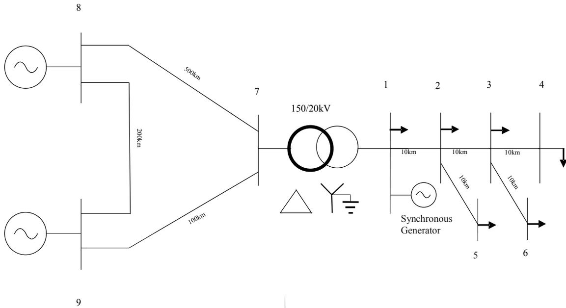
Fig. 6: Single-line diagram of 9-bus system [21].
