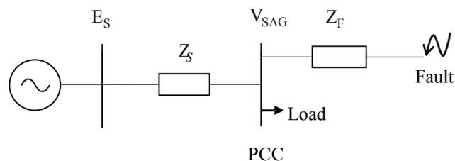
Fig. 1: Radial network supplying a sensitive load.
