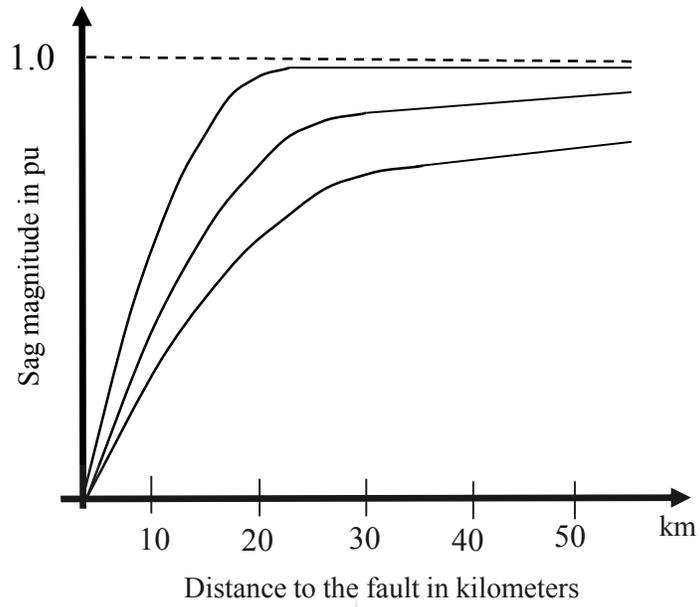
Fig. 2: Sag magnitude as a function of distance.
