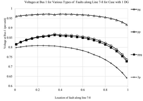
Fig. 10: Magnitude of voltage sag on the faulted phase recorded at bus 1 for faults on line 7-8 for Base Case and DG Case.
