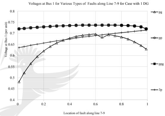
Fig. 11: Magnitude of voltage sag on the faulted phase recorded at bus 1 for faults on line 7-9 for Base Case and DG Case.
