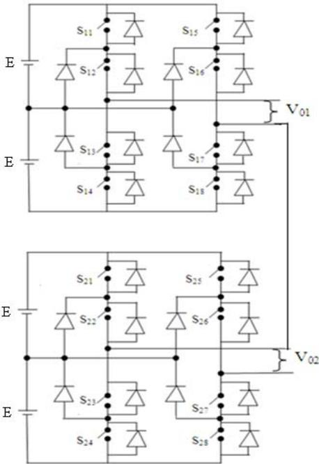
Fig. 1. Topology of a nine-level cascaded NPC/H-bridge inverter
