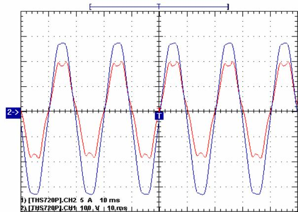
Figure 5. Oscilloscope results showing phase voltage and Current with compensation of 28.3  $\mu\text{F}$  under full load conditions, the current is distorted with Total Harmonic Distortion of 8.6 % due to the 5<sup>th</sup> and 7<sup>th</sup> harmonics.
