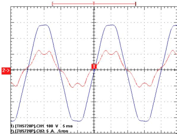
Figure 6. Oscilloscope results showing phase voltage and Current with compensation of  $28.3 \mu\text{F}$  at half load, the current is highly distorted with Total Harmonic Distortion of 16.2 % due to the 5<sup>th</sup> and 7<sup>th</sup> harmonics.
