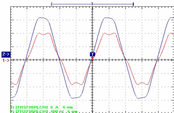
Figure 4. Oscilloscope results showing phase voltage and Current with compensation of 30  $\mu\text{F}$  at full load conditions, the current is distorted with Total Harmonic Distortion of 8.5% due to the 5<sup>th</sup> and 7<sup>th</sup> harmonics.
