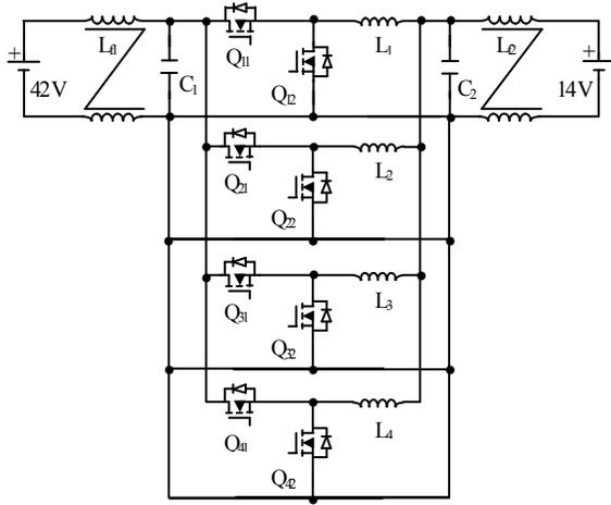
Fig. 4 Interleaved bi-directional dc/dc converter
