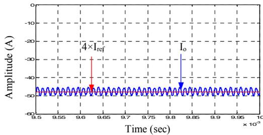
Fig. 14 Output current for interleaving in buck mode
