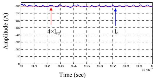
Fig. 15 Output current for interleaving in boost mode
