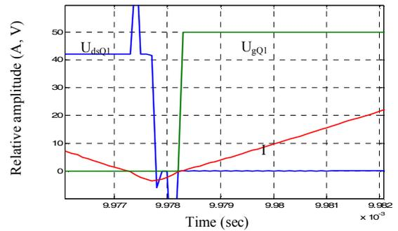
Fig. 12 Zero voltage for the lower transistor  $Q_1$
