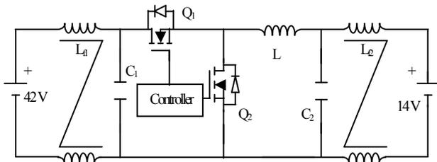
Fig. 3 Basic topology of the bi-directional dc/dc converter
