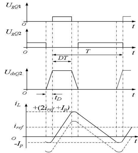
Fig. 5 Gating pulses; drain voltage and current through inductance  $L$
