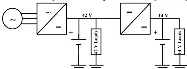
Fig. 1 Block diagram of the dual voltage system
