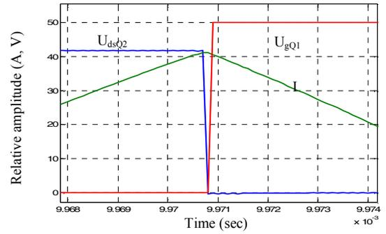
Fig. 11 Zero voltage for the lower transistor  $Q_2$
