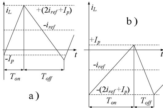
Fig. 6 The current waveform through inductance  $L$ : a) in buck mode; b) in boost mode.
