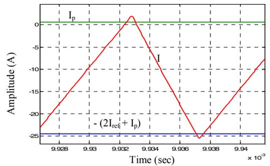
Fig. 13 Inductor current for  $I_{ref} = 12$  A in boost mode
