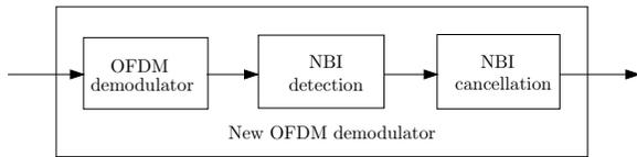
Fig. 8. New OFDM Demodulator.
