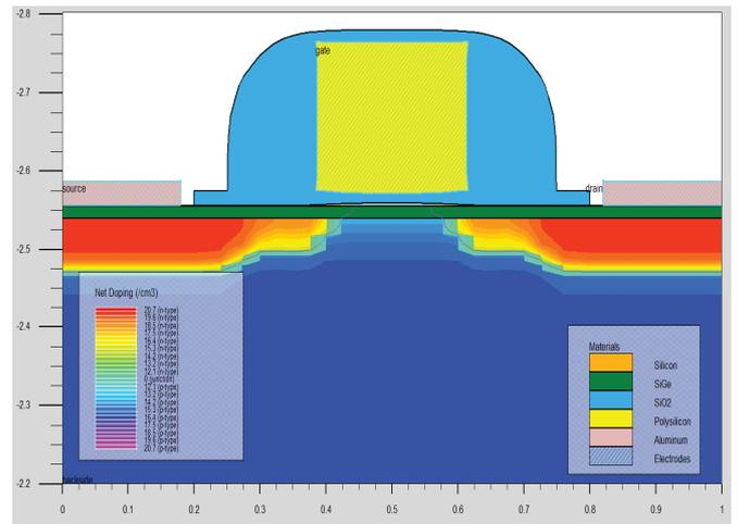
Fig. 3. Complete Structure of Biaxial Strain NMOS Silicon
