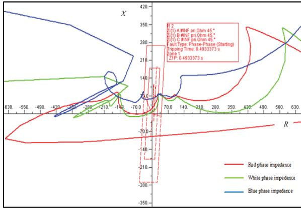
Figure 12: Trajectory impedance seen by the relay 2
