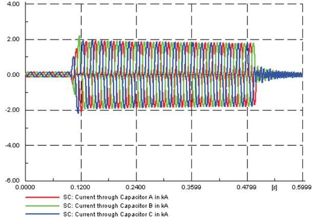
Figure 16: Current flowing through the capacitor bank
