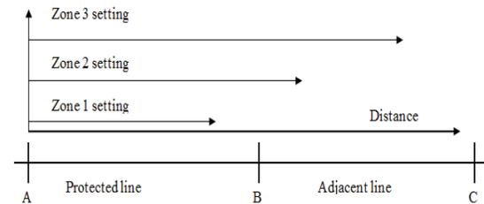
Figure 7: A typical distance protection settings
