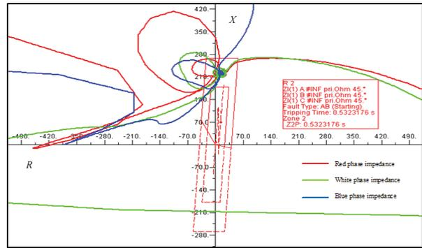
Figure 10: Trajectory impedance seen by the relay 2
