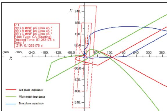
Figure 9: Trajectory impedance seen by the relay 1
