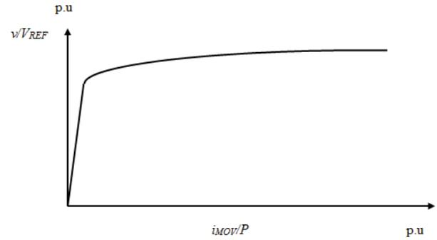
Figure 5: Voltage- Current characteristics of the MOV
