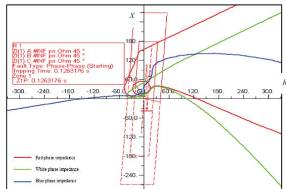
Figure 11: Trajectory impedance seen by the relay 1
