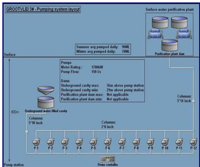
Figure 4: Layout of Grootvlei 3 shaft pump station
