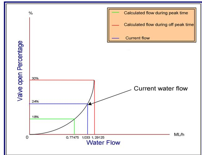
Figure 9: 27 level plug valve % opening and flow rate
