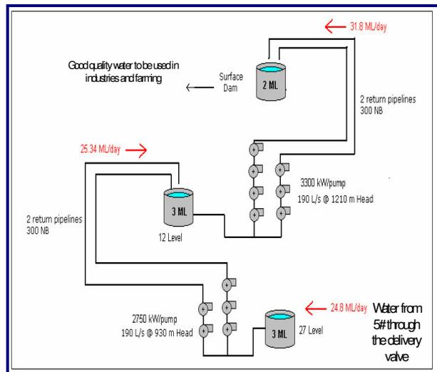
Figure 6: Kloof 10 shaft pump system layout
