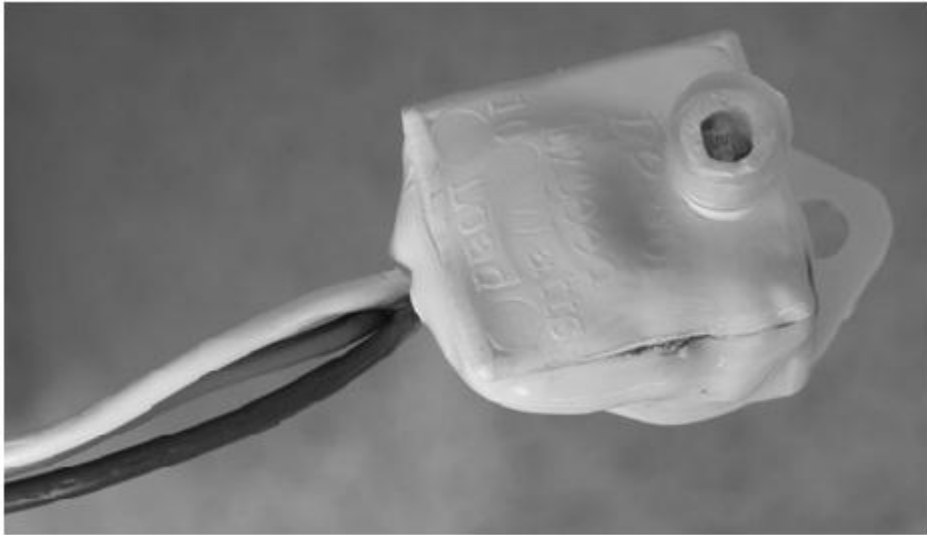
Figure 10: Switch Overheated by CFL Load
