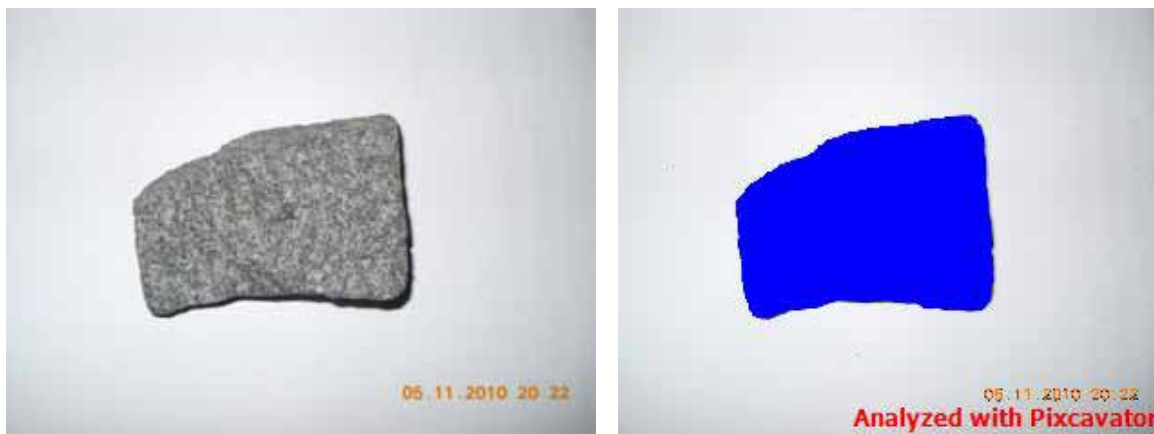
Figure 7: A dolerite ballast image that has been analyzed using the pixcavator (Method 2)
