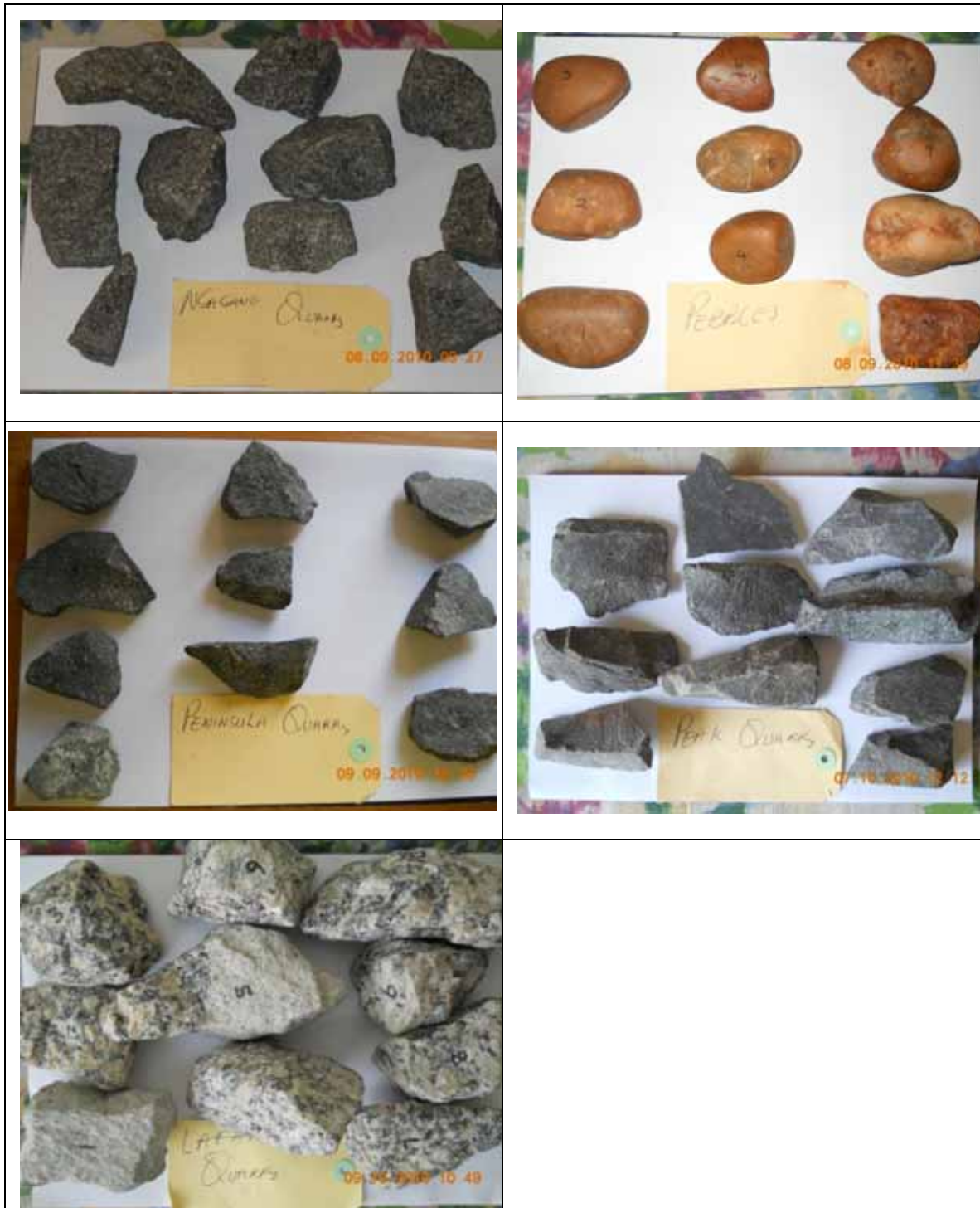
Figure 1: The different types of ballasts samples for the project: 1. Newcastle Dolerite; 2. Kimberley Pebbles; 3. Peninsula Greywake; 4. Worcester Shale; and 5. Saldanha Granite
