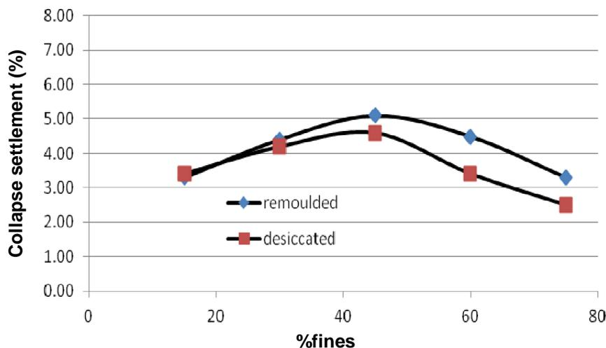
**Figure 6.** Collapse settlement curve of desiccated and remoulded samples of Johannesburg quartzite at at normal stress of 200 kPa, moisture content of 7% and dry density of 1580 kN/m<sup>3</sup>.
