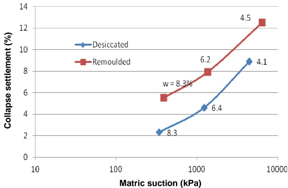
**Figure 8.** Collapse settlement – matric suction curves of Johannesburg quartzite compacted to dry density of 1450 kN/m<sup>3</sup> and inundated at normal stress of 200 kPa.
