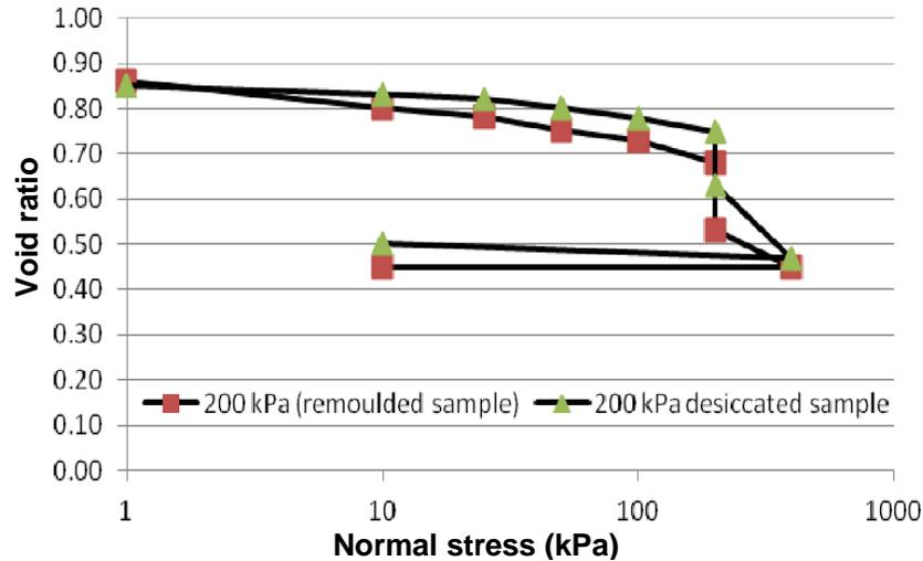
**Figure 3.** e-Log<sub>p</sub> graphs of desiccated and remoulded samples of Johannesburg quartzite at normal stress of 200 kPa and moisture content of 7% and dry density of 1580 kN/m<sup>3</sup>.
