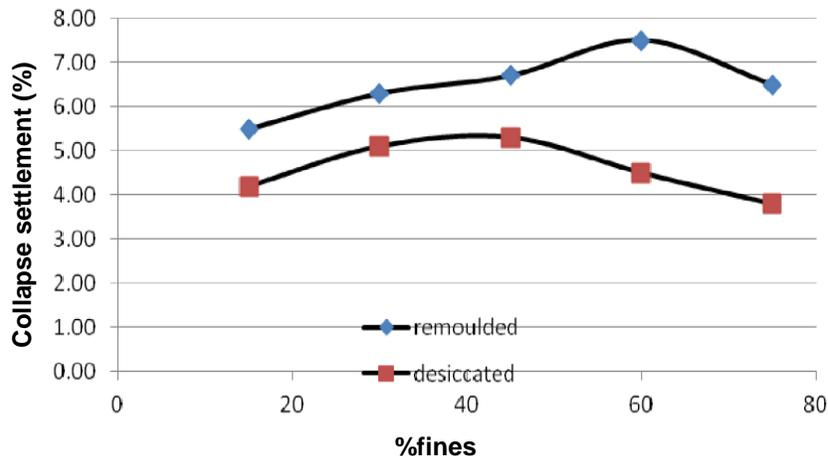
**Figure 5.** Collapse settlement curve of desiccated and remoulded samples of residual quartzite at at normal stress of 200 kPa, moisture content of 7 % and dry density of 1450 kN/m<sup>3</sup>.
