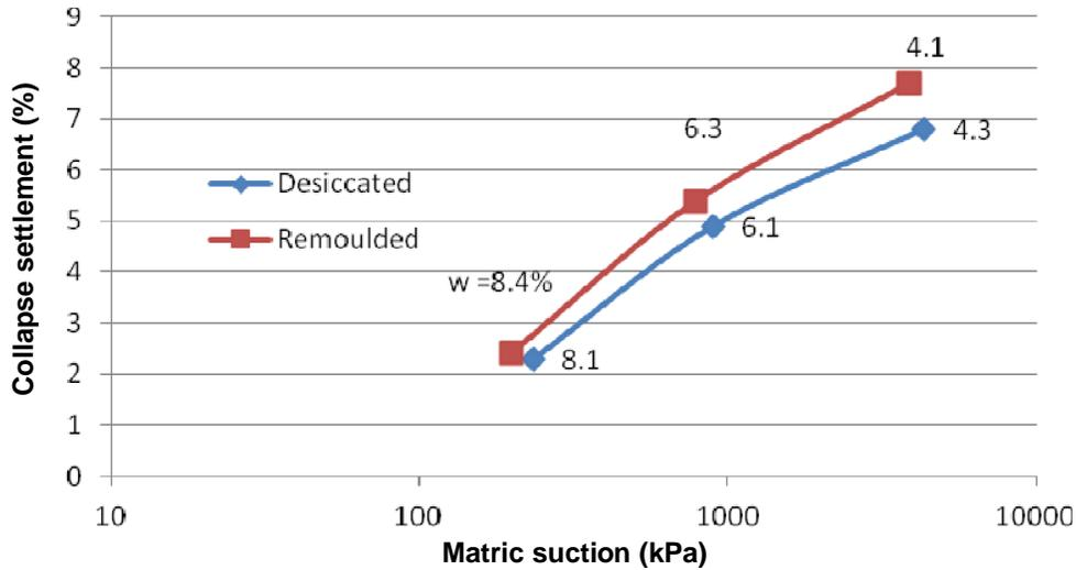
**Figure 7.** Collapse settlement – matric suction curves of Johannesburg quartzite compacted to dry density of 1450 kN/m<sup>3</sup> and inundated at normal stress of 400 kPa.
