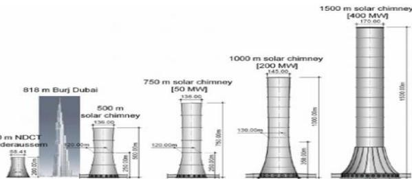
Figure 4: Heights of Solar Chimneys' and power outputs.
