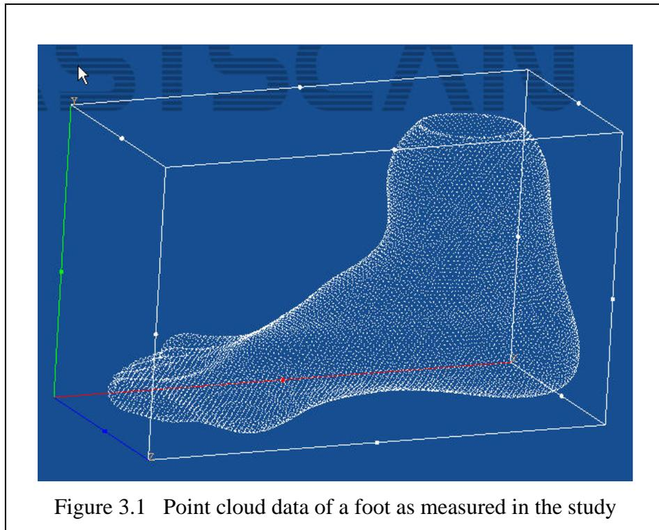
Bearing in mind industry's future needs for contour data, the ability to capture point cloud data became an important criterion in the investigation to select a 3-D data input method.
