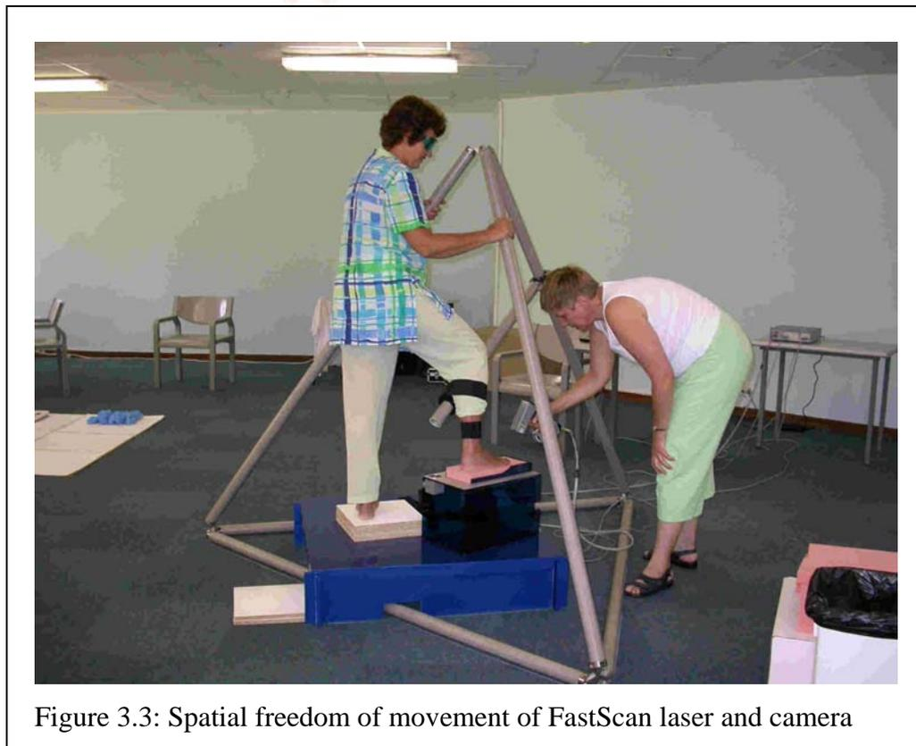
Figure 3.3: Spatial freedom of movement of FastScan laser and camera
