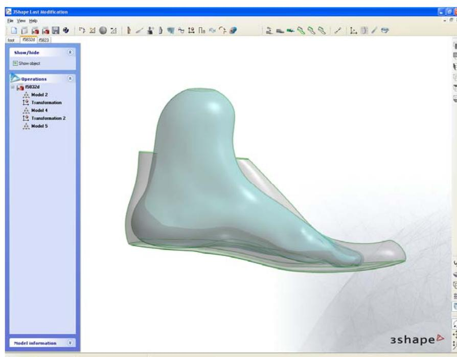
Figure 5.5: Digital comparison of foot data set to a model last
