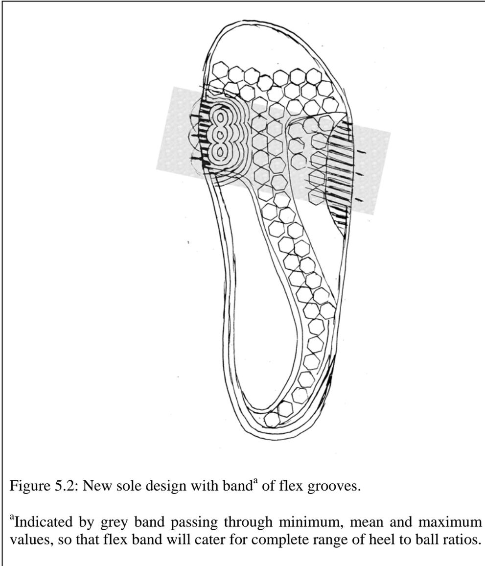
Figure 5.2: New sole design with band<sup>a</sup> of flex grooves.
