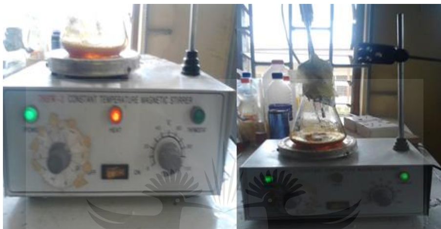
Figure 3.2: Transesterification setup of alcoholysis of Parinari polyandra seed oil
