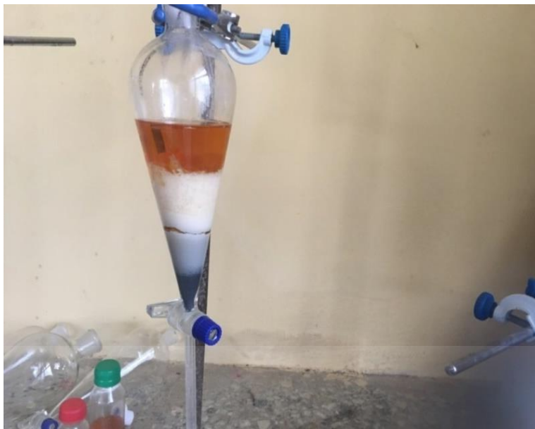
Figure 4.2: Settling phase of ethyl ester and glycerol
